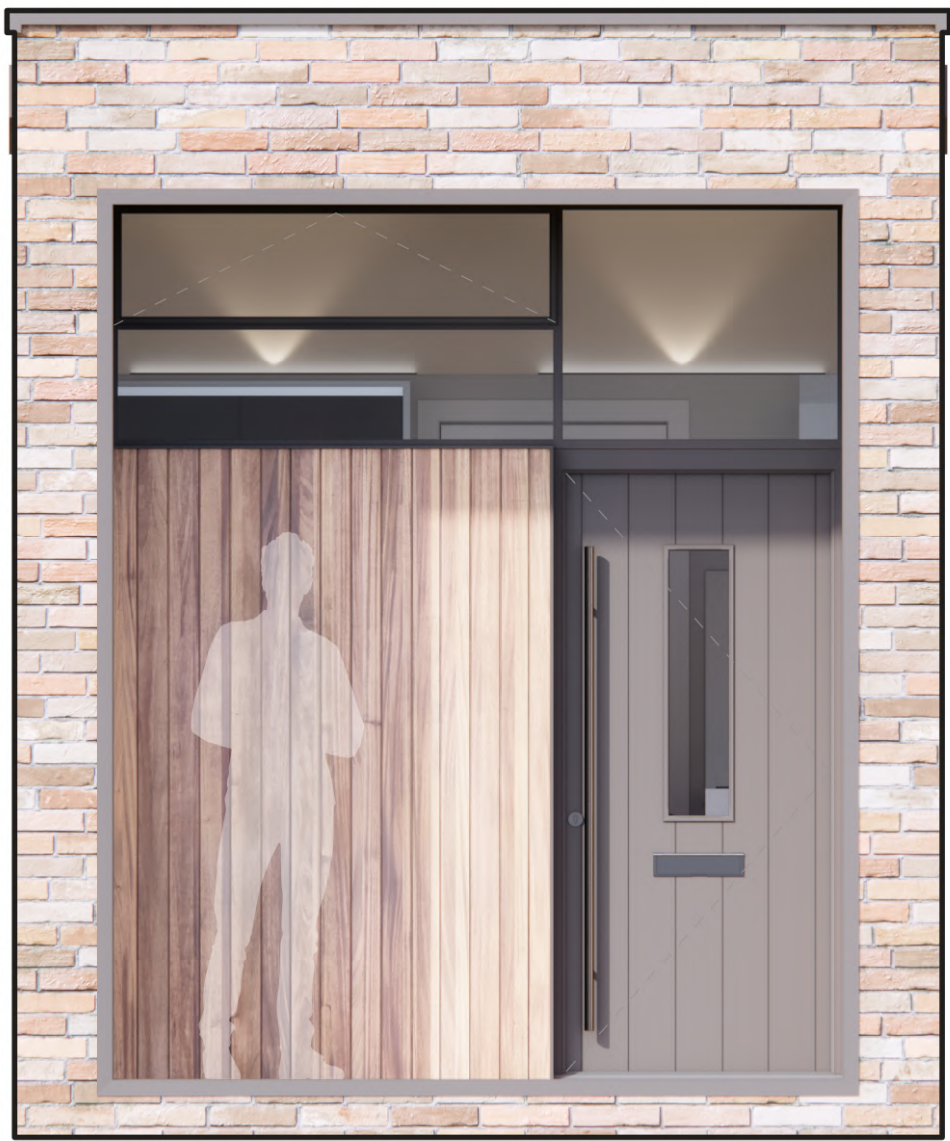
Front Elevation - Brick Slip
