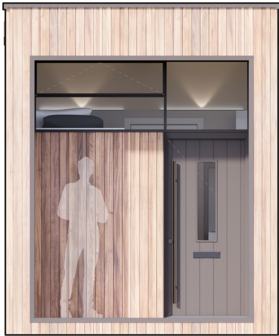
Front Elevation - Timber / Weather Board Cladding
